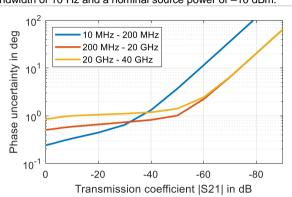
Uncertainty of transmission magnitude and transmission phase measurements for the R&S $^{\odot}$ ZNB40 model .72 in the frequency range from 10 MHz to 40 GHz; analysis conditions:  $S_{11} = S_{22} = 0$ , cal. power -10 dBm, meas. power -10 dBm
