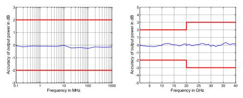
Output power accuracy in dB versus frequency for the R&S®ZNB40 model .82 and .84
