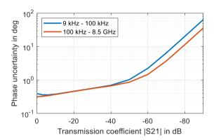
Uncertainty of transmission magnitude and transmission phase measurements for the R&S $^{\circ}$ ZNB4 in the frequency range from 9 kHz to 4.5 GHz, for the R&S $^{\circ}$ ZNB8 in the frequency range from 9 kHz to 8.5 GHz; analysis conditions:  $S_{11} = S_{22} = 0$ , cal. power -10 dBm, meas. power -10 dBm
