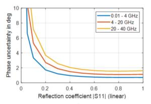
Uncertainty of reflection magnitude and reflection phase measurements for the R&S $^{\circ}$ ZNB40 model .72 in the frequency range from 10 MHz to 40 GHz; analysis conditions:  $S_{12} = S_{21} = 0$ , cal. power -10 dBm, meas. power -10 dBm
