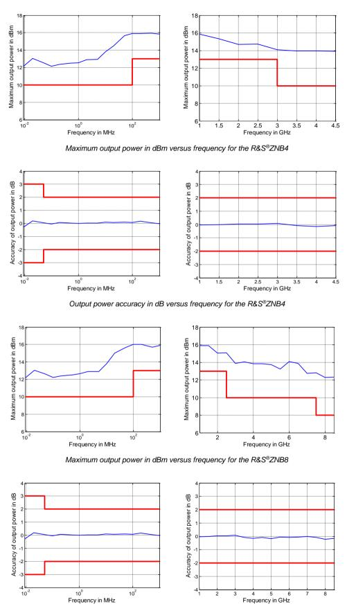
Output power accuracy in dB versus frequency for the R&S®ZNB8
