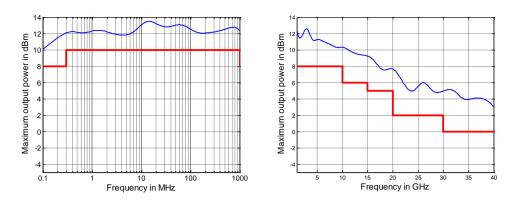
Maximum output power in dBm versus frequency for the R&S®ZNB40 model .82 and .84
