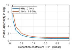
Uncertainty of reflection magnitude and reflection phase measurements for the R&S $^{\circ}$ ZNB4 in the frequency range from 9 kHz to 4.5 GHz, for the R&S $^{\circ}$ ZNB8 in the frequency range from 9 kHz to 8.5 GHz; analysis conditions:  $S_{12} = S_{21} = 0$ , cal. power -10 dBm, meas. power -10 dBm
