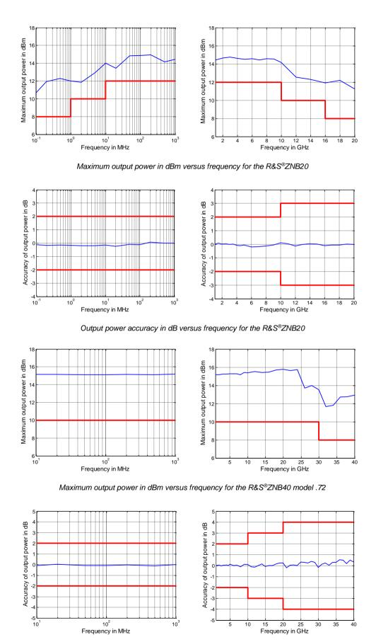
Output power accuracy in dB versus frequency for the R&S®ZNB40 model .72
