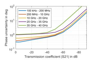
Uncertainty of transmission magnitude and transmission phase measurements for the R&S<sup>®</sup>ZNB40 model .82 and .84 in the frequency range from 100 kHz to 40 GHz; analysis conditions:  $S_{11} = S_{22} = 0$ , cal. power –10 dBm, meas. power –10 dBm
