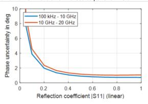
Uncertainty of reflection magnitude and reflection phase measurements for the R&S®ZNB20 in the frequency range from 100 kHz to 20 GHz; analysis conditions:  $S_{12} = S_{21} = 0$ , cal. power -10 dBm, meas. power -10 dBm
