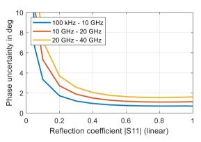
Uncertainty of reflection magnitude and reflection phase measurements for the R&S $^{\odot}$ ZNB40 model .82 and .84 in the frequency range from 100 kHz to 40 GHz; analysis conditions:  $S_{12} = S_{21} = 0$ , cal. power –10 dBm, meas. power –10 dBm
