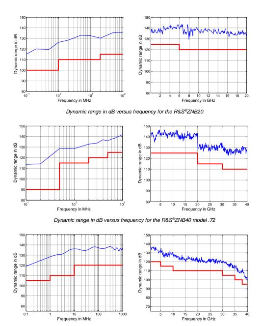
Dynamic range in dB versus frequency for the R&S®ZNB40 model .82 and .84
