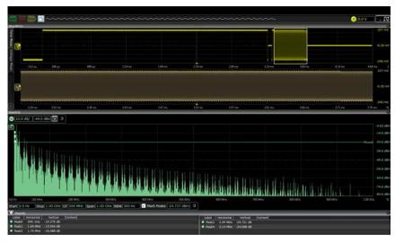
The UXR-Series FFT quickly identifies peaks and has key controls such as span, start and stop, which make the oscilloscope behave more like a spectrum analyzer
