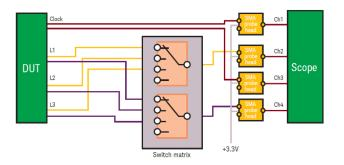
Typical switch configuration for HDMI testing
