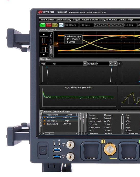
Up to 100x faster performance for some measurements – enabled by a powerful new measurement acceleration ASIC and memory controller capable of 5 trillion integer operations per second (IOPS)
