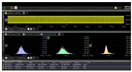
With its flat frequency response and low noise, the UXR-Series is able to accurately measure jitter components such as ISI.
