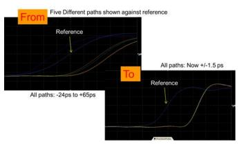
Skews between switch paths are easily maintained with Keysight's unique Infiniium software
