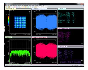
Never before seen 64 Gbaud 256 QAM 1-Tb/s coherent modulation analysis with 2.6% EVM – made possible by the Infiniium UXR-Series real-time oscilloscope and its world's lowest noise, 110 GHz of bandwidth, 256 GSa/s sampling, high-definition 10-bit ADC and industry best ENOB
