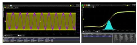
With 110 GHz bandwidth and a 256 GS/s sample rate, the UXR-Series is able to effectively characterize the time interval error trend of high-speed signals as well as fast rising edges, down to 2.8 ps.
