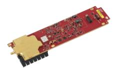
Dual-channel 33 GHz MCM and single-channel 110 GHZ MCM with integrated faraday cage heat sink
