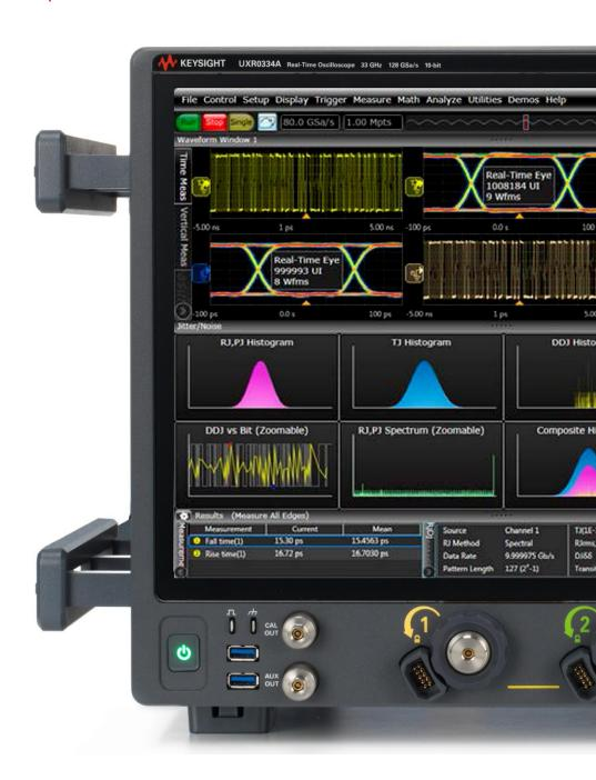
Threaded 3.5 mm RF connectors with convenient auto torque mechanism ensures the most reliable signal integrity and consistent 8 in-lbs connection. The AutoProbe II interface provides a robust interface and instant compatibility with the InfiniiMax III and III+ probing system.
