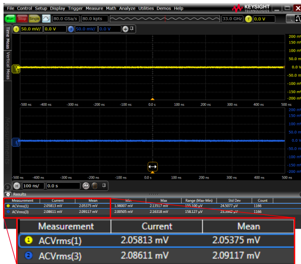
Ultra-low noise at 33-GHz full bandwidth (2.10 mV at 50 mV/div).
