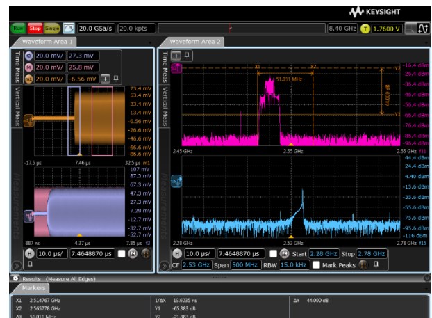
Perform measurements in the area of interest through the gated function.
