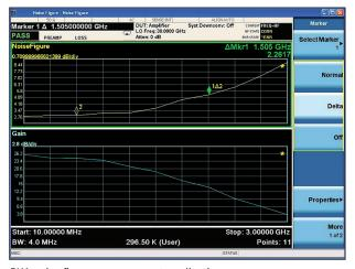
PXA noise figure measurement application
