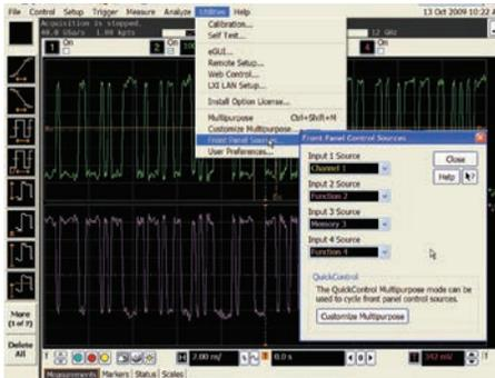
Ever wanted to change the scale or offset of a function or waveform memory? If you have, you know that it requires multiple menus and key strokes. In Infiniium software version 2.01 and later, you can now map functions and waveform memories to the front panel controls of the oscilloscope!
