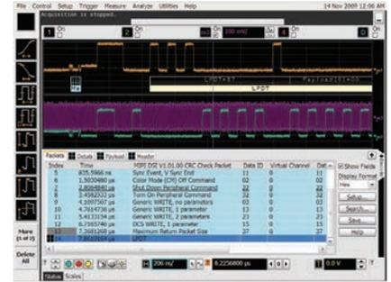
Trigger on and decode MIPI packets.
