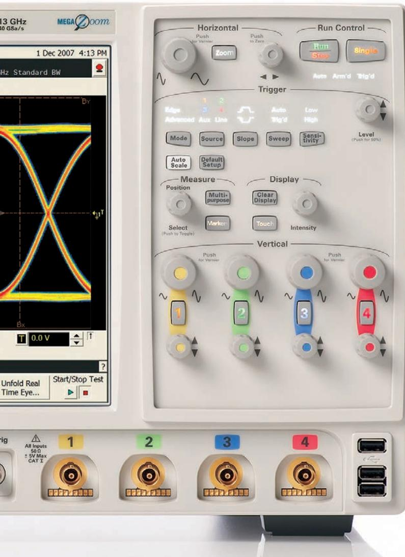
Simply press the **horizontal delay knob** to set the delay value to zero. A zoom button provides quick access to two screen zoom mode.
