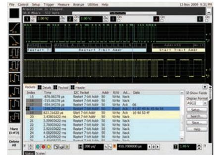
Trigger and view on-screen serial decode of I<sup>2</sup>C packets.
