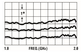
Center trace is phase response of 8491A -6 dB attenuator from 1.0 to 2.0 GHz taken with the 8410 network analyzer. Top and bottom traces are  $\pm 1^{\circ}$  calibration. Linear phase component has been compensated for with a line stretcher. Response, therefore, shows nonlinear phase deviation of  $< \pm 1/2^{\circ}$  over 1 to 2 GHz band.
